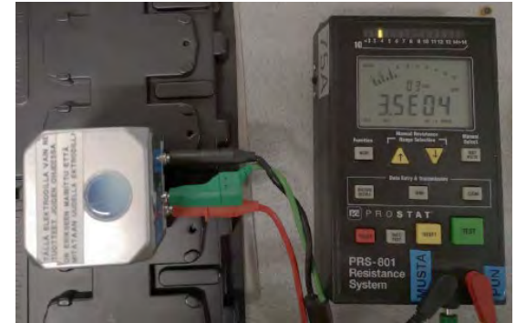
Vacuum formed sample from the bottom, more strain -> higher resistance
