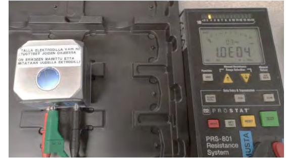
Vacuum formed sample from the middle, less strain -> lower resistance
