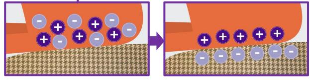
Mr. Statix's backside is rubbing the car seat. He becomes positively charged.
